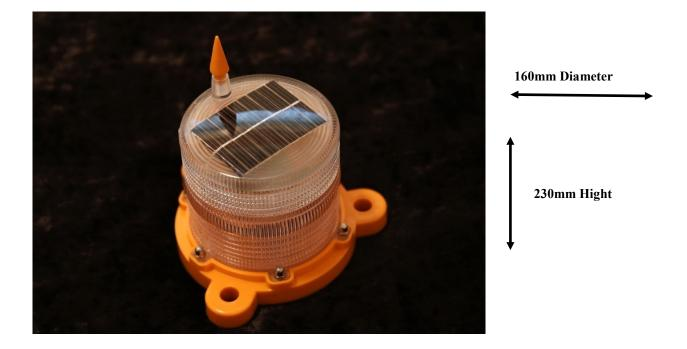
Available in hook or spike Working Temperature is -25 to +75 Degrees C Contains 2 x Ni-MH 1.2V/1200mAH Batteries 8 x super bright LED`s Waterproof IP68 Grade Luminous mode: Constant or Flashing Work Time with no light 130 hours flashing Poly Carbonate Construction Solar Cell Single-Crystalline Silicon Available in Amber, Red, Blue Green
