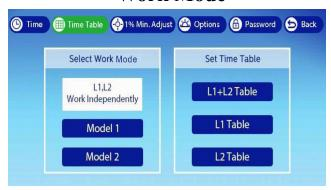
Model 1 will allow both output lines to work as the same. (the 2000 watt controller has only 1 output unless specified.)
