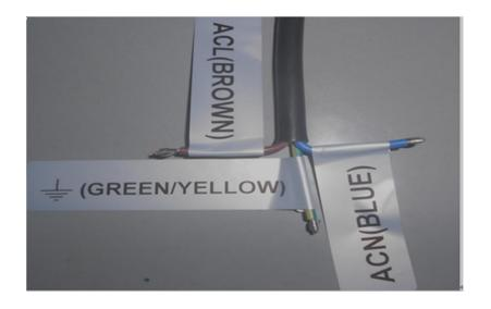
ACL: Connect the Brown input ACN: Connect the Blue input
