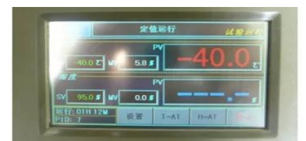
Temperature Chamber -40~60°C working test
