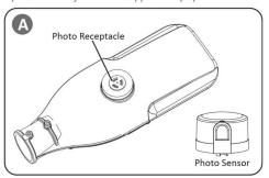
If the fixture has PHOTO CONTROL function, the Photo Receptacle will be installed on the cover of fixture. Fit the pins of Photo Sensor to Photo Receptacle, firmly insert and rotate Photo Sensor to proper position.
