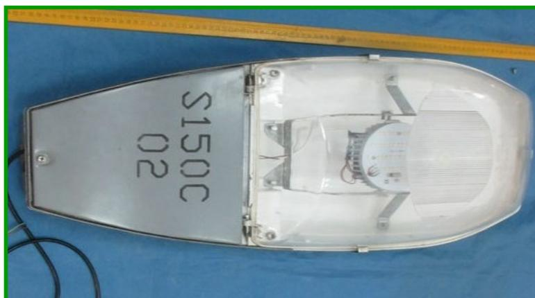
**Step 12.** Check for dust or any foreign objects & clip original lens cover into position ensuring there is a good seal & clips are in good working order.
